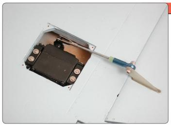
Once the glue has fully cured fit the aileron servo with self tapping screws as shown and make up the pushrod and install. Note that for security the servo extension lead should be taped to the servo lead when they are plugged together.
