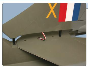
Fit the fin/rudder, connecting the rudder extension lead to the servo lead at the same time – secure the connection with wrap of tape or similar. Note that the carbon mounting rods fit down through the tailplane and into the mountings in the fuselage.
